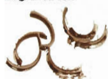
Chips produced when cutting above part of 4140 material using new Rigid-Lock XR roughing ball nose endmill.
