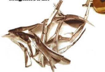
Chips produced when cutting above part of 4140 material using standard finishing ball nose endmill.
